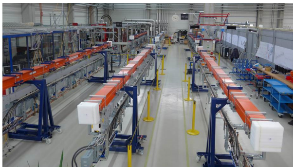
Figure 3: Five assembled module waveguide distributions at WATF.
