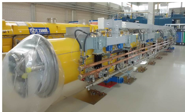
Figure 4: Module waveguide distribution connected to one accelerator module.
