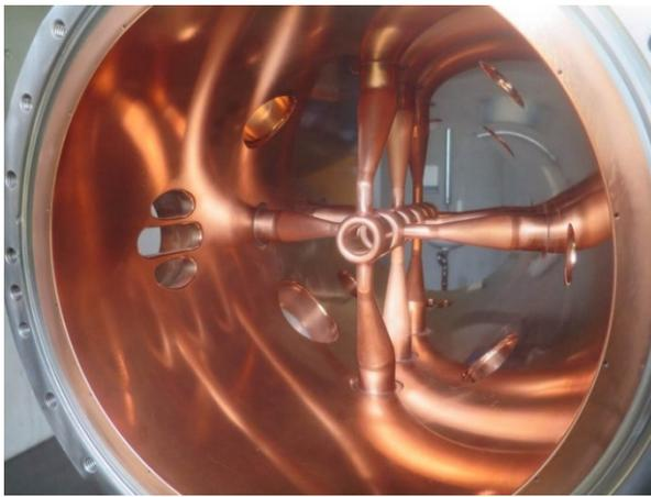
Figure 2: CH cylindrical tank after the copper plating.
