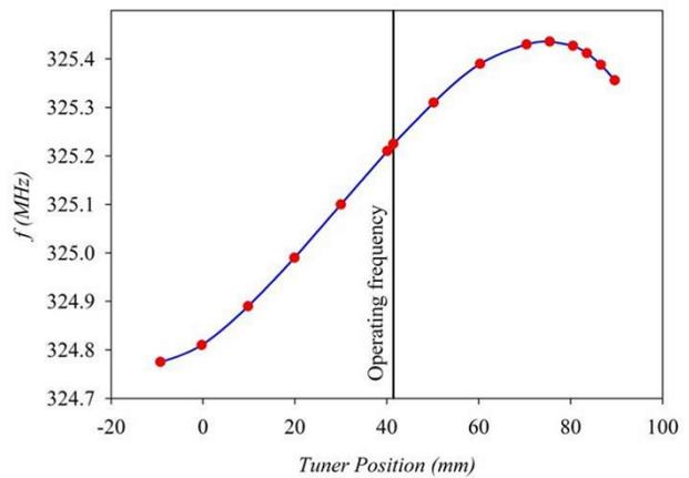
Figure 4: Tuner frequency shift of the movable tuner versus the tuner position.
