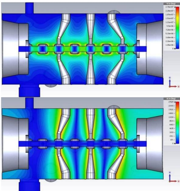
Figure 3: Electric (top) and magnetic (bottom) fields.
