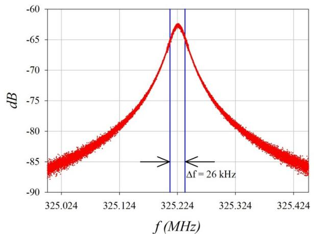
Figure 5: Resonance frequency and quality factor measurements.
