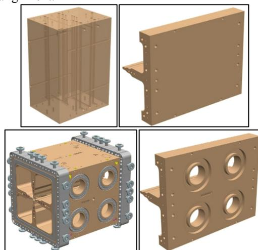
Figure 1: Component geometries along the production phases: 1 ,2, 3,7 (clockwise, from top left).
