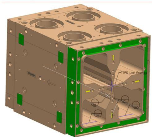
Figure 3: Dry assembly module with some element reference use for the module reference coordinate system.
