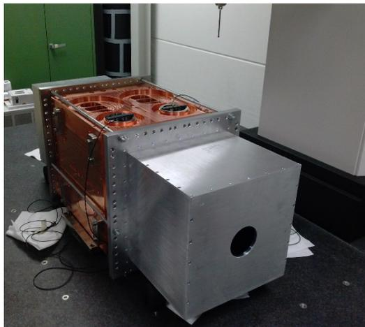
Figure 5: A RFQ module connected with the square waveguide for RF measurements
