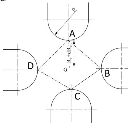
Figure 4: Beam axis point G calculated based on the transversal TIPS profile measured.
