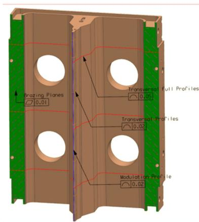
Figure 2: Form tolerances applied on curves of significant 3d-curve surfaces.
