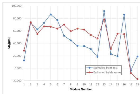
Figure 6: Average  $\Delta R_0$  estimation for each RFQ module. The red curve represents the outcome of mechanical measurements, while the blue curve represents the outcome of RF measurements.
