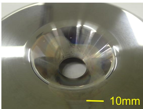
Figure 2: The photograph of the existing wehnelt electrode.
