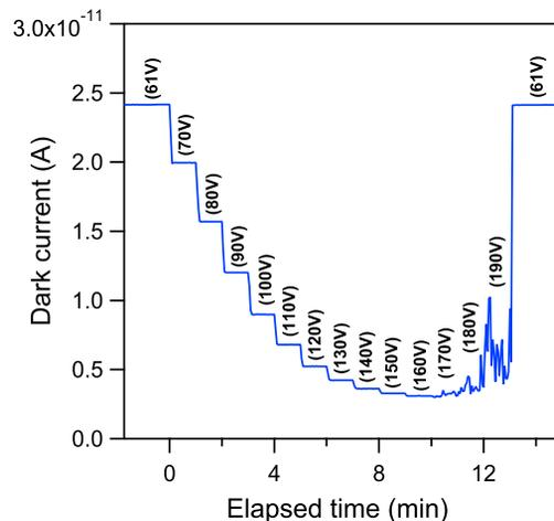
Figure 3: Dark current as a function of elapsed time at various bias voltages for the cathode with the new electro-polished anode and wehnelt electrodes. Elapsed time was set to be zero min when bias voltage of the cathode started to increase from 61V. Cathode heater voltage was 6.00V. Bias voltages for the cathode were expressed in parentheses.
