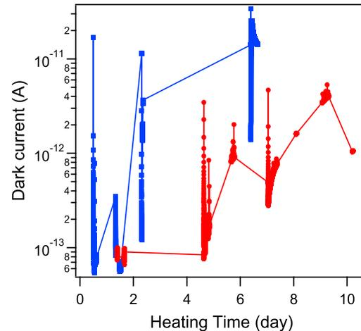
Figure 5: Heating time dependence of dark current from the improved electron gun and from the improved electron gun using the existing Y-845 cathode assembly under the same operating condition as the real accelerator. Red lines with circle markers and blue lines with rectangle markers represent dark current from the improved electron gun and the improved electron gun using the existing Y-845 cathode assembly, respectively.
