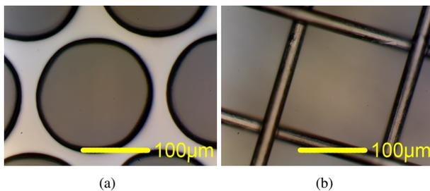
Figure 4: Optical microscope images of the grid electrodes of (a) the newly-developed and (b) the existing Y-845 cathode assemblies.
