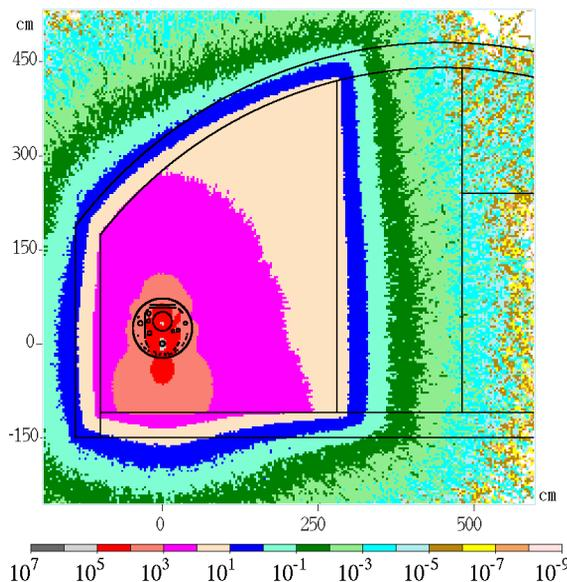
Figure 1: Total prompt dose (mSv/hr, color scale) at the tunnel cross section at the end of ILC linac during normal operation. Focusing magnet strength corresponds to 250 GeV beam.
