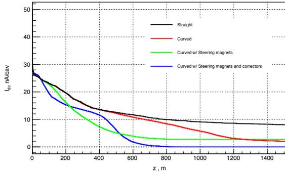
Figure 2: 50 nA DC from a single cavity at the beginning of 1.5 km linac section of 40 RF units with focusing magnets turned off. Different colors show distributions for 4 different scenarios: straight section (black), curved section (red), curved section with steering magnets (green), and curved section with correctors and steering magnets (blue).
