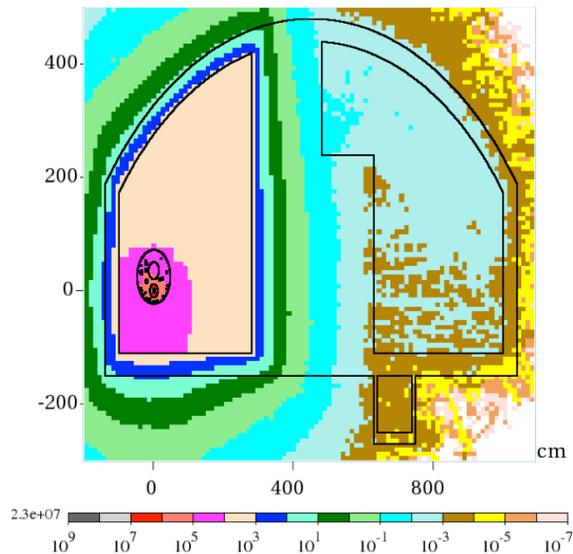
Figure 5: Total prompt dose (mSv/hr, color scale) at the tunnel cross section for the equilibrium DC losses in a curved section of randomly misaligned linac with steering and corrector magnets turned on.
