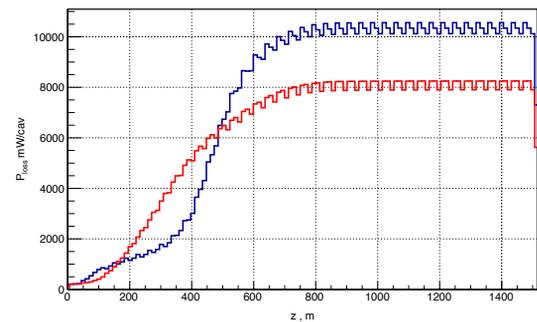
Figure 4: Power loss of DC electrons per cryo-module in the curved section of linac with steering magnets turned on and correctors off (red) or on (blue). All cavities contribute 50 nA.
