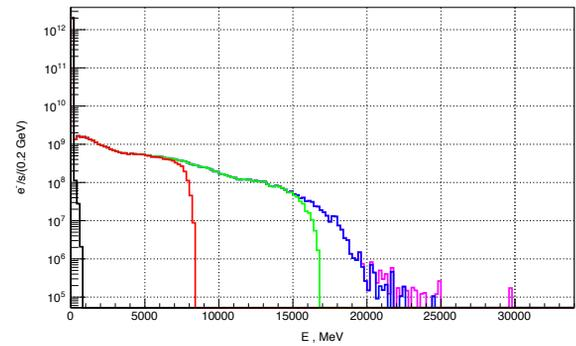
Figure 3: Energy distribution of lost particles in a single unit in a curved section of linac of 40 RF units with correctors and steering magnets turned on. All cavities contribute 50 nA DC. Different colors show distributions for unit 1 (black), unit 10 (red), unit 20 (green), unit 30 (blue), and unit 40 (magenta).
