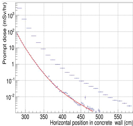
Figure 6: Distribution of prompt dose in the tunnel wall. Set of data points at the lower curve corresponds to normal operation of linac. Upper set of points corresponds to operation with focusing magnets turned off and steering and correcting magnets turned on.
