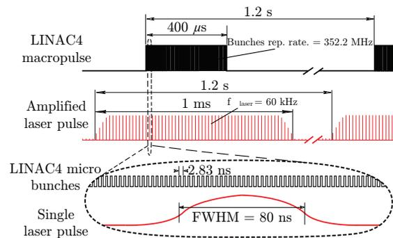
Figure 5: Timing of Linac4 and laserwire compared [6].
