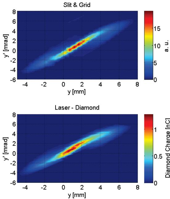
Figure 7: Phase-space sampled with the slit/grid method (top), with the laser/diamond system (bottom) [7].
