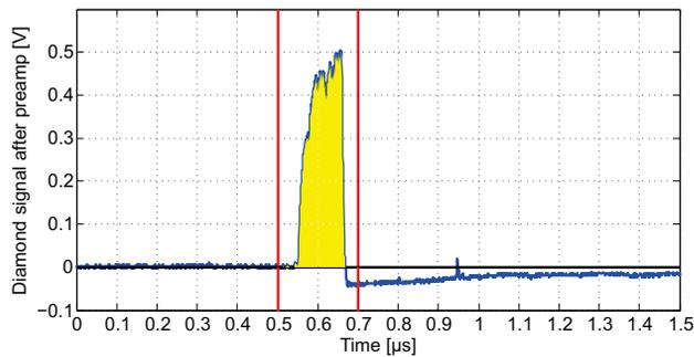
Figure 10: Signal of liberated electrons as measured by the diamond detector with integration limits in red and integrated charge in yellow.
