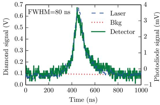
Figure 6:  $H^0$  pulse on the diamond detector (solid - inverted), compared to the corresponding laser pulse (dashed). Dotted trace – linear fit of the background [6].
