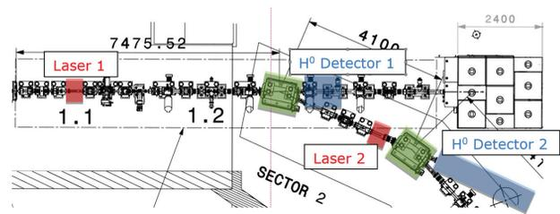
Figure 12: Setting for 2 laserwire instruments, which will be installed at the 160 MeV region at Linac4.
