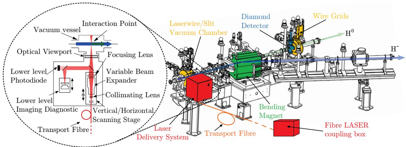
Figure 2: Layout of the 3 and 12 MeV diagnostics test-bench, including the operational emittance meter (slit and grid) and the laserwire emittance scanner prototype [6].
