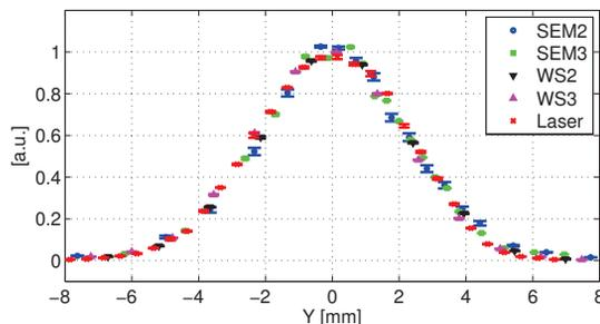
Figure 11: Overlay of profiles recorded at 107 MeV energy with different devices (WS = wirescanner; SEM = Secondary Emission Grid).
