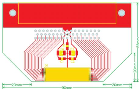
Figure 15: Design of diamond detector used for  $H^0$  detection at 160 MeV.
