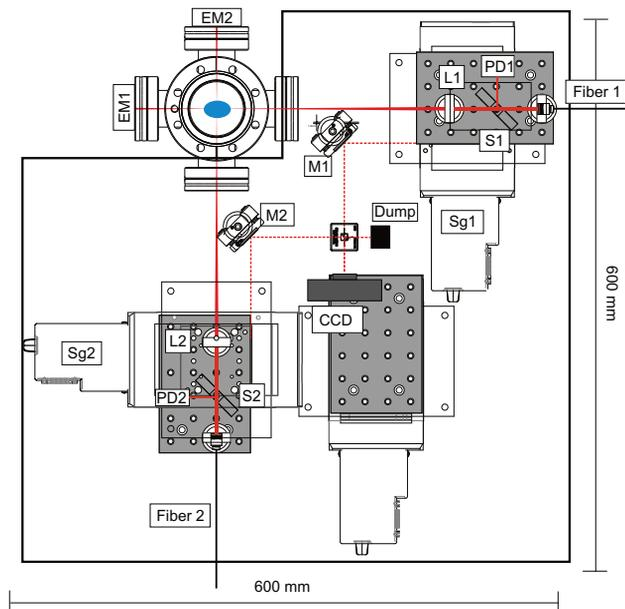
Figure 13: Laser injector with beam-pipe.
