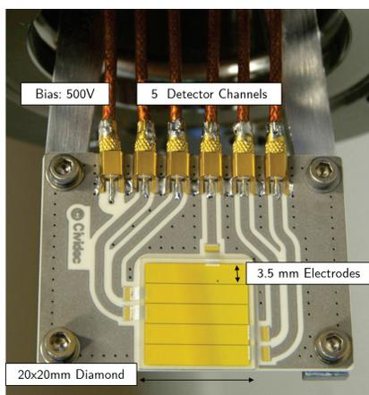
Figure 4: pCVD diamond detector with 5 strip electrodes [6].
