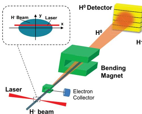
Figure 3: Concept for combined vertical profile and emittance measurement. Measurement in the horizontal plane can be realized by rotating the laser beam and the  $H^0$  strip-detector by  $90^\circ$ .
