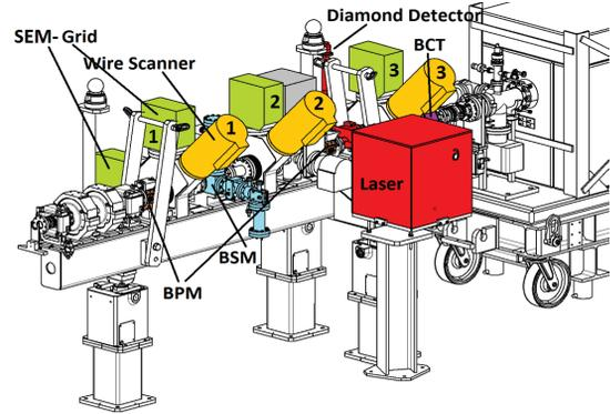
Figure 8: Diagnostic test-bench used for beam commissioning at 50, 80 and 107 MeV  $H^-$  beam [8].
