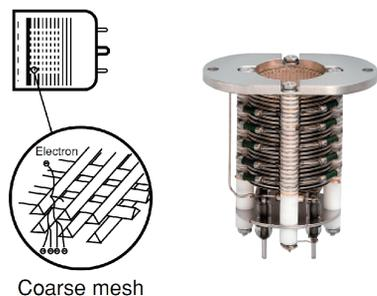
Figure 14: Electron Multiplier Tube (EMT). Left: Principle of coarse mesh type EMT; Right: Photo of EMT selected for 160 MeV electron detection [11, 12].
