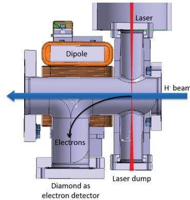
Figure 9: Setup for profile measurement. Detached electrons are deflected by a weak dipole field and recorded by a sCVD diamond detector [9].
