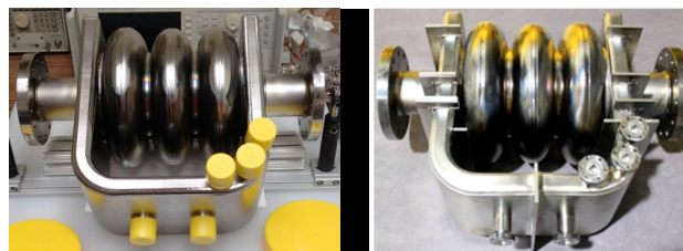
Figure 1: 3-Cell traveling wave cavity with (right) and without (left) stiffening ribs on the waveguide.
