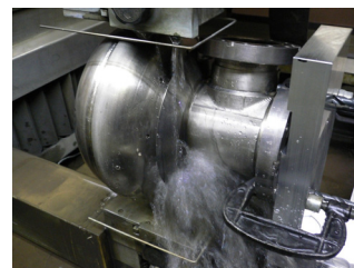
Figure 2: Removal of the end plate with an EDM.
