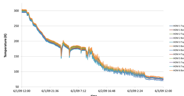
Figure 2: Typical cool-down profile of the ICM using the initial heat exchanger can. Rather huge transients can be seen as well as oscillations on the cooldown from nitrogen to helium temperatures.
