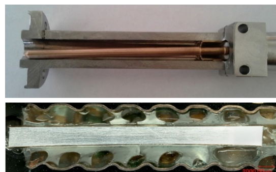
Figure 2: Sections of damaged coupler and RF cable after stress test in vertical cryostat.
