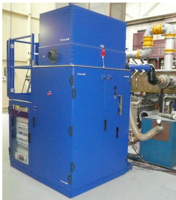
Figure 1: New 1.8 MW cavity amplifier prototype after factory acceptance tests at THALES.
