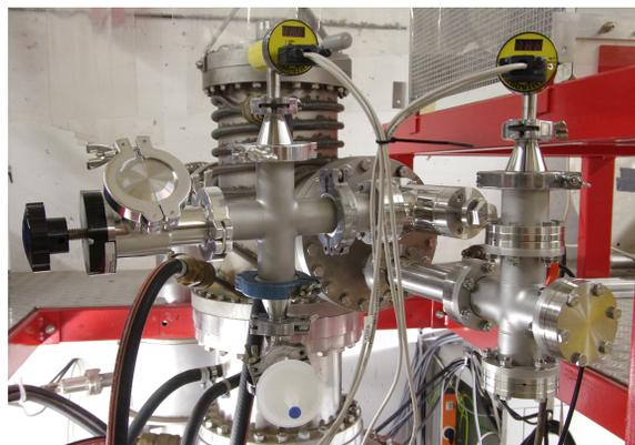
Figure 6: Nitrogen supply system at the top of the furnace. As only a small volume is required, it consists of a KF40 cross in the center with attached periphery: At the top a Pirani vacuum gauge, on the left a vacuum valve for a vacuum pump, at the bottom a nitrogen inlet with particle filter. On the top right is a additional Pirani vacuum gauge to monitor the pressure inside the hot-pot.
