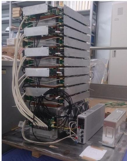
Figure 3: Solid-state switch using SI thyristors.
