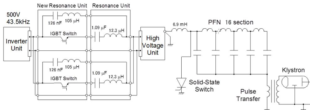
Figure 1: Circuit diagram of the klystron modulator.
