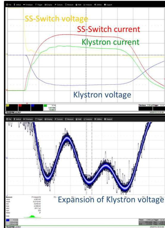
Figure 4: Voltage and current waveforms of klystron and solid-state switch and expansion of the klystron voltage.
