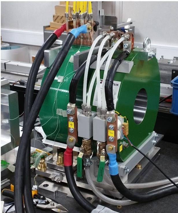
Figure 4: Magnetic system of the gun on the test stand.
