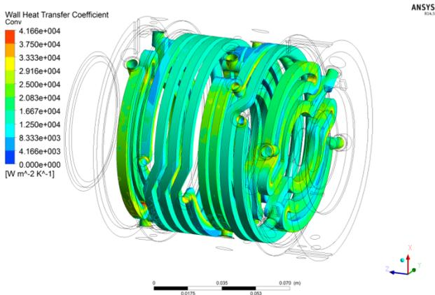
Figure 1: Wall convective heat transfer coefficient in High Repetition Rate Gun cavity as calculated with the ANSYS CFX technique.
