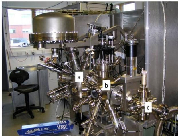
Figure 3: Photocathode Preparation System. a-Analysis Chamber, b-Preparation Chamber, c-Transport Vessel.
