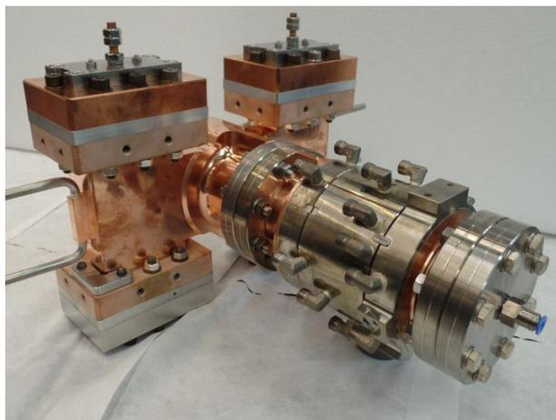
Figure 2: HRRG cavity after manufacturing.
