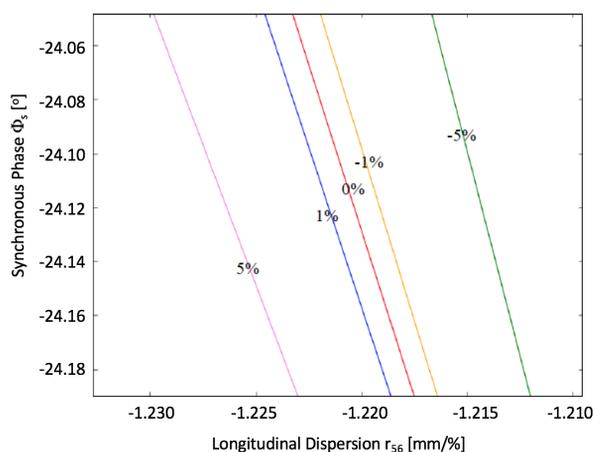
Figure 5: Magnified region of fig. 4 (right) indicating a line of perfect energy recovery (0% energy deviation). By slight variation of the synchronous phase one is able to find optimum performance.
