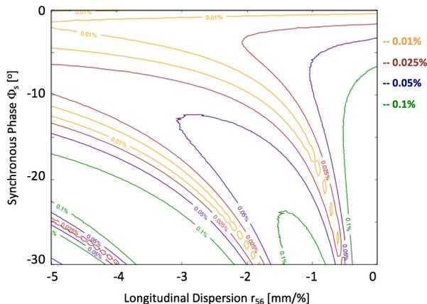
Figure 2: Hill plot of the energy spread as a function of longitudinal dispersion and synchronous phase after 5 linac accelerations. The lowest energy spread is  $3.9 \cdot 10^{-5}$  for  $r_{56} = -3.4$  mm/% and  $\Phi_s = -17.1^\circ$ , more than a factor of 2 in reduction compared to  $8.3 \cdot 10^{-5}$  for the isochronous/ on-crest case ( $r_{56} = 0$  mm/%,  $\Phi_s = 0^\circ$ ).
