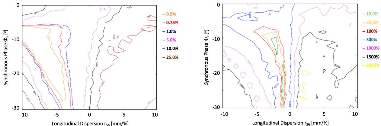
Figure 4, left: energy spread of the highest energy beam as a function of the longitudinal working point assuming only path length variations of 5 mm. Right: energy deviation from the injection energy after energy recovery. A 0% deviation means full energy recovery. This plot indicates that a working point which is minimizing the energy spread at full energy leads to poor energy recovery efficiency and vice versa.
