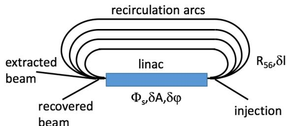
Figure 1: Recirculating linac/energy recovery linac scenario calculated within this paper.  $R_{56}$  and  $\Phi_s$  are the parameters under which the linac and the arcs are operated.  $\delta A$  and  $\delta\phi$  are the jitters that are applied to the cavity fields and  $\delta l$  is the random path length variation.
