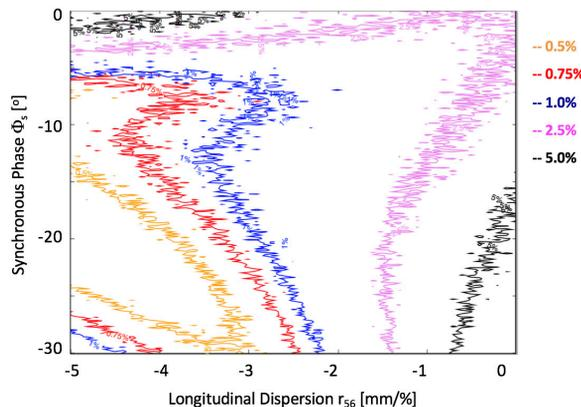
Figure 3: Hill plots of the energy spread as a function of  $r_{56}$  and  $\Phi_s$ . This calculation was performed applying RF jitters and random path length variations between  $\pm 5$  mm.
