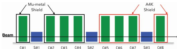
Figure 1: Layout of FRIB-1 Cryomodule (CM-1). C: cavity (green); S: solenoid package (blue). Cavities 1–4 are shielded by mu-metal (black) and Cavities 4–8 are shielded by A4K (red).
