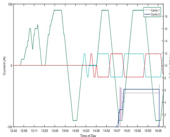
Figure 5: Coil currents as a function of time for part of the solenoid tests in CM-2. The two adjacent cavities were turned on between 15:08 and 16:06.
