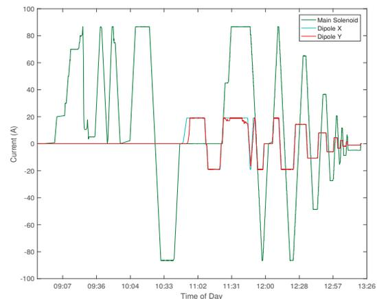
Figure 4: Coil currents as a function of time for part of the solenoid tests in CM-1.
