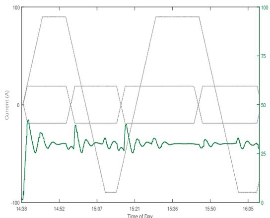
Figure 6: Example of PID control while ramping the solenoid current at 0.3 A/s. The set point is a voltage drop of 30 mV.
