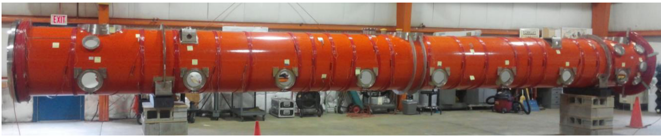
Figure 6: Helmholtz coils on the exterior surface of the LCLS-II pCM vacuum vessel [3, 9].
