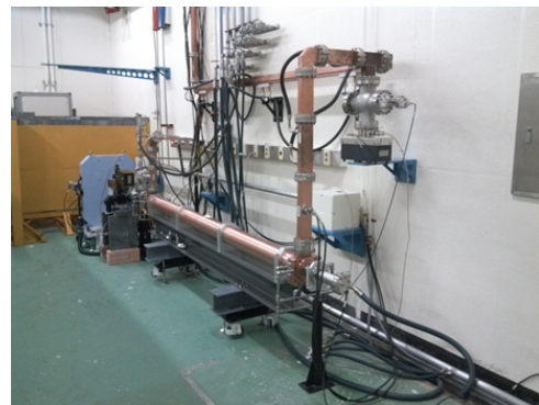
Figure 6: Accelerator column high power test setup at ATF.
