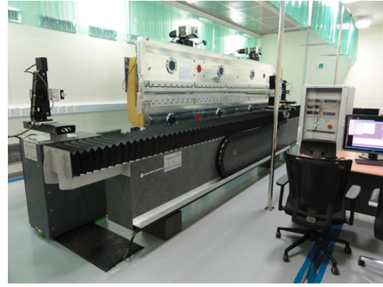
Figure 9: Insertion device test laboratory (top) and field measurement set-up of the undulator prototype (bottom).
