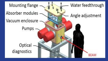
Mechanical schematic of a 50-Ohm kicker Test of a 150-W amplifier as a kicker driver: output signal for a single pulse MEBT absorber: TMZ alloy, 40 cm long. Requirements: 21 kW beam, ~2mm rms rad, 29 mrad grazing angle.
