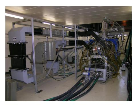
High power RF conditioning of the TRASCO RFQ
