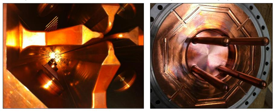
Traces of discharge on vane tips high energy part (low field region) and on high energy termination plate
