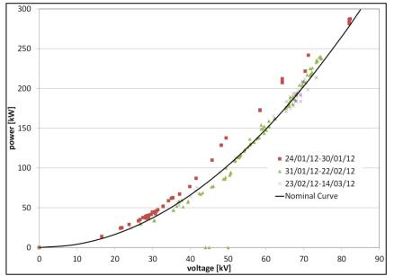
High power RF conditioning of the TRASCO RFQ
