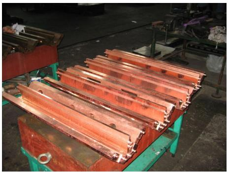
Major and minor vanes under fabrication: cooling water channels have been drilled and the ends have been plugged.
