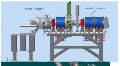
A Penning H- ion source and a three-solenoids LEBT with space charge neutralization. Pre-chopper is mounted at the entrance of the RFQ with a beam rise time of 15ns.
