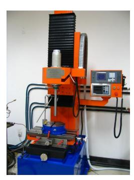
A new rotating-coil measurement system so as to reach a high accuracy of 0.006mm and high efficiency in the measurement of the magnetic center.
