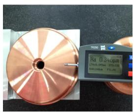
The tank is made of carbon steel and the inner surface is copper-plated, with a thickness of 0.15mm after polishing. Full copper drift tube has very good surface machining.
