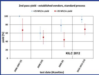
International cavities from established vendors using established processes 2<sup>nd</sup> pass yield for >35 MV/m for integrated sample is (57 +- 8)% for 2010-2012 alone is (69 +- 13)% Ginsburg LINAC12
