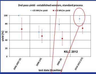
International cavities from established vendors using established processes 2<sup>nd</sup> pass yield for >25 MV/m for integrated sample is (80+- 7)% for 2010-2012 alone is (92 +- 7)% Ginsburg LINAC12
