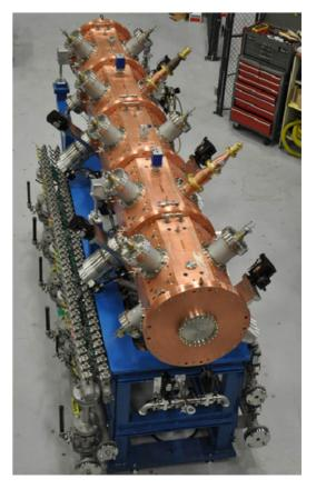
Figure 1: Completed RFQ assembly.
