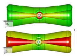
Figure 5: A half-wave resonator model in MWS. The electric (top) and magnetic field (bottom) distributions on the surface are shown.
