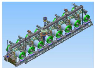
Figure 6: PXIE HWR cryomodule design
