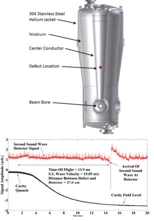
Figure 1: (Top) The cavity with a red dot placed at the height of the defect in the center conductor, the cavity is 53 inches from top to bottom . (Bottom) A single quench event with an oscillating superleak transducer signal and the cavity transmitted power.
