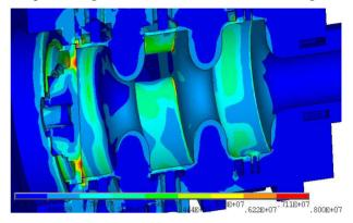
Figure 8: Thermal stress (N/m<sup>2</sup>) for a 0.9 kW average load on the SwissFEL RF gun body.
