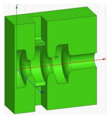
Figure 2: Cross-section of the SwissFEL RF gun.
