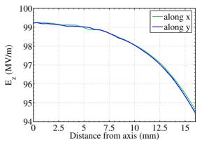
Figure 4: Amplitude of the longitudinal electric field along transverse directions of the SwisFEL RF gun.
