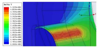
Figure 5: Coupling aperture temperature rise for a 3  $\mu$ s RF pulse and a peak on-axis field of 100 MV/m.
