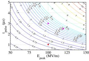
Figure 7: Average dissipated power (kW) vs. peak accelerating field and pulse length for a repetition rate of 100 Hz.
