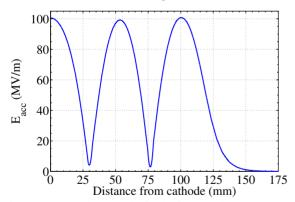
Figure 3: On-axis electric field of the SwisFEL RF gun.
