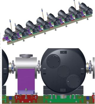
Figure 2: (Top) A cavity/solenoid string mounted on a strong-back. (Bottom) A close up of the alignment hardware for a solenoid and a cavity. The runners move transversely by adjusting two screws which push and two screws which pull (screws not shown but threaded holes they mate with are). One of each adjustment type is on each corner. The runners can be moved up and down by adjusting two vertical screws and placing shims between it and the strong-back.
