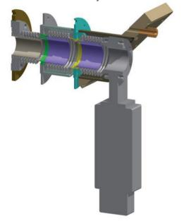
Figure 5: Cross section view of the beam-line gate valve. The total heat leak to 2 K in this design is < 0.05 W. For the 4 K cryomodules the final bellows segment on the left will be removed.
