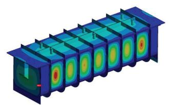
Figure 1: ANSYS results of the vacuum vessel deformation due to a 14.7 psi static pressure gradient across the walls. The red color corresponds to displacements greater than 0.6 inches with the maximum being 0.67 inches.
