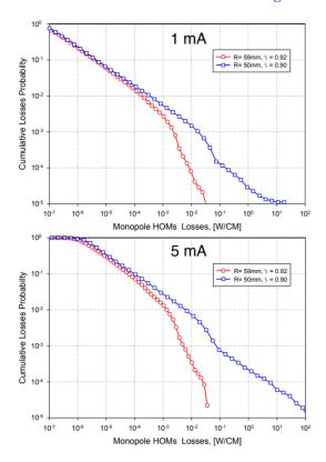
Figure 6: Probability of power loss per cryomodule for the monopole HOMs for the present (blue) and alternative (red) HE cavities.
