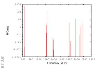
Figure 4: (R/Q) of the monopole HOMs in PX HE section.
