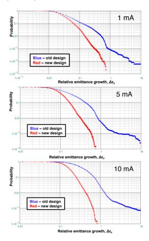
Figure 7: Probability of longitudinal emittance growth in the HE section of PX linac for 1 mA (top), 5 mA (middle), and 10 mA (bottom) average beam current. Data for the present design of the cavity are shown in blue, data for the alternative design are in red.
