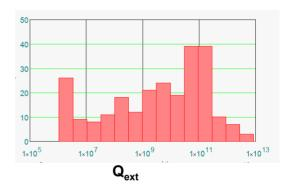
Figure 5: Variation of  $Q_{ext}$  for the monopole HOMs in the  $5^{th}$  passband of HE cavity.
