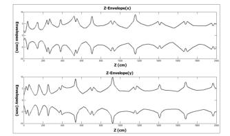
Figure 3: The x and y transverse envelope along the linac.
