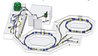
Figure 1: The whole HIRFL-CSR Layout with CSR-LINAC injector.
