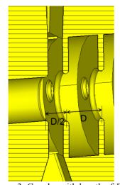
Figure 3: Coupler with length of D/2.
