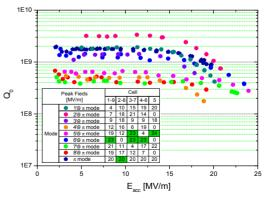
Figure 3:  $Q_0$  vs  $E_{acc}$  for all fundamental pass-band modes of cavity 3HZ03. The mode analysis shows that cells #2 and #8 are limiting the cavity performance in the  $\pi$  mode, while the other individual cells reach 23 MV/m and above (values highlighted in green).
