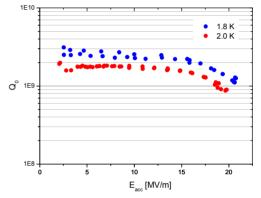
Figure 2:  $Q_0$  versus  $E_{acc}$  for cavity 3HZ03 at 2.0 K and 1.8 K. The cavity is quench limited without X-ray or field emission.
