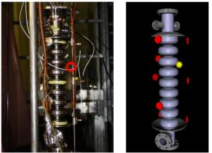
Figure 4: OSTs around the cavity (left photograph of the cavity in the insert) and reconstruction of the quench origin (model on the right). The source is highlighted by the red circle on the left and represented by the yellow sphere on the right, where OSTs are shown in red.
