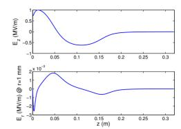
Figure 4: Field distribution  $(E_z, E_r)$  of a 1.4 cell gun cavity design with 35 mm exit iris and 53 mm beam tube radius.
