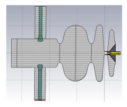
Figure 5: Possible design of the next 1.4 cell gun cavity featuring the HZDR-style choke cell, a modified cathode stock, two TTF-III type FPC having a 35 mm exit iris.
