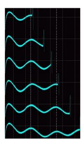
Figure 5: Rf signal modulation at 50 Hz (reflected power, left) and 1 Hz (phase difference forward/reflected, right) pulse repetition rate for pulse lengths of appr. 2-6 ms.
