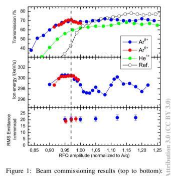
Figure 1: Beam commissioning results (top to bottom): Transmission, ion energy and beam emittance for different ions as a function of the rf amplitude, normalized to the mass-to-charge ratio. Reference data: Old RFQ; dashed line: Derived working point.
