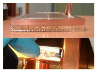
Figure 2: Tuning plate with burnt contact springs (top) and new contacts (bottom). The thick silver foil is pressed against the stem by spring steel foil and steel wedges.
