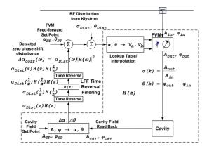
Figure 3: Time reversal filtering for FVM error detection
