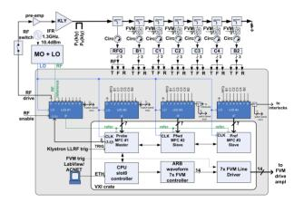
Figure 1: LLRF system configuration
