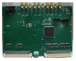
Figure 3: The timing extension hardware
