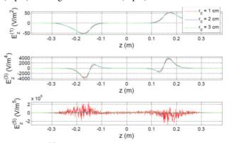
Figure 4:  $E_z^{(n)}(z)$  of n=1, 3 and 5 at  $r_0=1$  cm, 2 cm and 3 cm for the cylindrical-shaped 400 MHz rf-dipole cavity.
