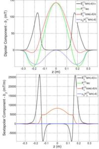
Figure 7: Dipolar and sextapolar field components of the 400 MHz cylindrical-shaped rf-dipole cavity.
