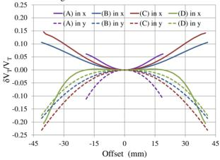
Figure 2: Normalized transverse voltage in x and y directions for designs (A), (B), (C) and (D) in Fig. 1.
