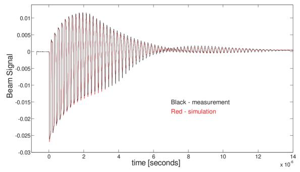
Figure 1: Excellent simulation/experiment agreement is seen in a comparison of the 6 mA wall-current monitor signal with simulated current profile adjusted to include beam loss and the equivalent circuit model of the detector.
