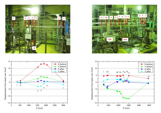
Figure 3: Beam duct realignment in MEBT2 (left) and ACS11 (right). Upper-left figure shows the section between MEBT2-QDM02 and MEBT2-QDM03 which have an IP in its center. Upper-right figure shows the ACS11 section which have a TMP in its center and a NEG Pump just before the TMP. Lower figures show the results of the duct position measurement before and after the duct realignment in MEBT2 (left) and ACS11 (right).
