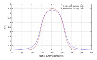
Figure 6: A solenoid with bucking coils has a lower fringe field in comparison with a simple solenoid. Both solenoids are normalized to the same focusing strength.
