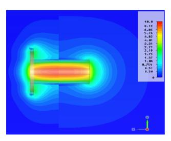
Figure 7: In this graphic two pictures with the magentic flux of a solenoid are merged. On the left side the solenoid with bucking coils is shown. The simple solenoid without bucking coils on the right side creates more spacious magnetic flux. The coloured scale is normalized to the highest field level of the left solenoid (4.5T). Both solenoids would have the same focusing strength, so the simple solenoid would have a less peak field (compare with figure 5).
