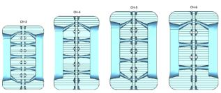
Figure 4: The four superconducting CH cavities in scale relatively to each other.
