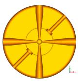
Figure 3: The diagonal tuners act mainly capacatively and provide a total frequency shift of 1 MHz.
