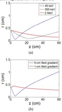
Figure 2: Beam envelop for (a) different injection energies, (b) two different lengths of field gradient at the DWA entrance for a 40-keV proton beam.
