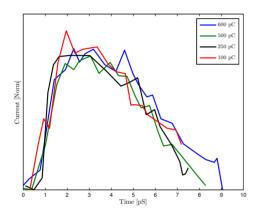
Figure 4: Temporal pulse profile of the e-beam bunch at different bunch charge levels. Pulse duration was approximately 5 pS for all experiments.
