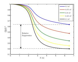
Figure 5: Noise suppression along the collective interaction region as calculated from solution of the coupled differential equations with  $\sigma_x(z)$ ,  $\sigma_y(z)$  of 70 MeV.
