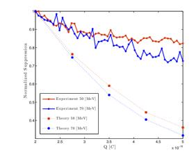
Figure 7: Relative noise suppression rate computed from Eq. 5 and 6 for E=50 MeV, 70 MeV compared to the experimental suppression results.
