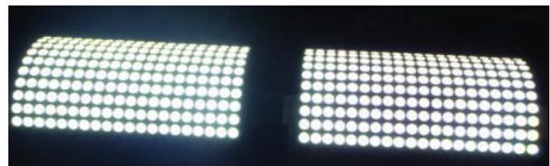
Figure 4: All the LED's are lighten. A diffusing panel will be install on the LED's to form the light strip. 14 chips/line x 2 lines/strip x 10 strips/side x 2 sides = 560 chips are used.
