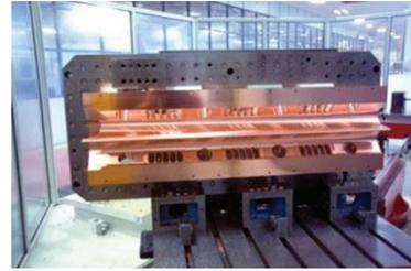
Figure 1 : Final machining of one RFQ's major vane
