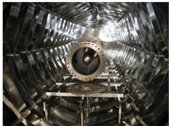
Figure 1: T-M Vacuum<sup>®</sup> high temperature vacuum furnace commissioned and being used to heat treat cavities at MSU.
