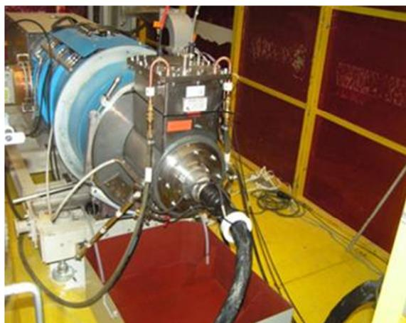
Figure 2: MBK with CM and HV cable “PFISTERER 3S”
