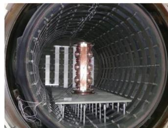
Figure 2: The RFQ in vertical position in the furnace
