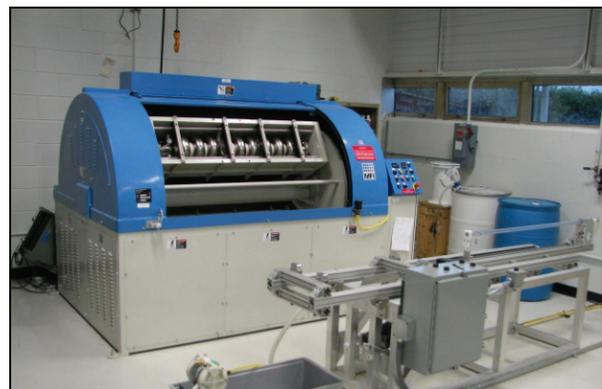
Figure 2: Centrifugal barrel polishing machine.
