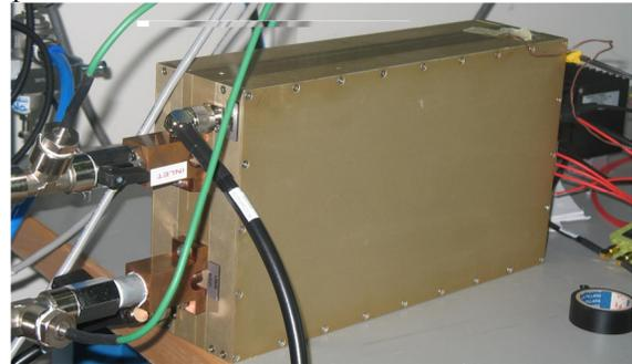
Figure 2: The double 800 W amplifier module view.
