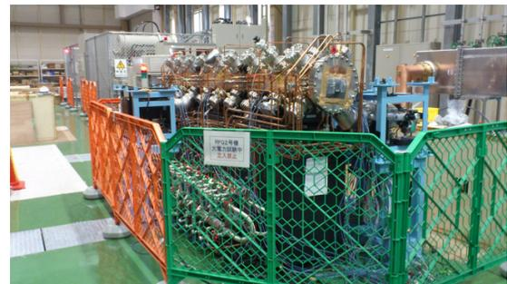
Figure 2: High-power testing RFQ II.
