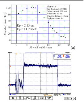
Figure 8: The beam testing results. Time-scale is 4 µs/division.
