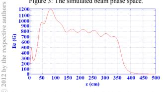
Figure 4: The solenoid magnetic field distribution along the 10 MeV / 40 kW linac.
