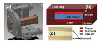
Figure 4: (a) 250 GHz structure mounted on a positioning holder; b) structure dimensions; c) photo of diamond after the experiment exhibiting no visible damage.
