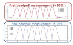
Figure 2: Bead-pulling RF measurement of first linac tank, showing good field balance across the cells.
