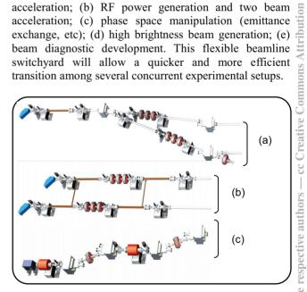
Figure 3: Different legs of the new AWA beamline switchyard will be dedicated to specific types of experiments: (a) collinear wakefield acceleration; (b) twobeam-acceleration and RF power generation; (c) phase space manipulation (emittance exchange) and beam diagnostic development.
