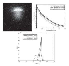
Figure 6: (top left)X-ray profile measured by EMCCD sheltered by 1.5cm silicon. (top right) Attenuation curves at points a, b, and c. (bottom) The reconstructed local X-ray spectrum from the attenuation curves.
