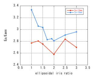
Figure 4: Ratio of maximum surface electrical field to the on-axis electric field  $(E_p / E_{acc})$  depending on the ratio of B/A.
