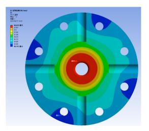
Figure 5: Temperature distribution of the accelerating structure in 120 pps operation
