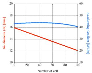
Figure 1: Variation of the iris diameters (red line/left axis) and an accelerating gradient at an input power of 80 MW (blue line/right axis).
