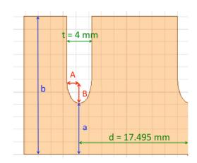
Figure 3: Cross sectional view of the ellipsoidal curved iris shape.
