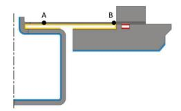
Figure 3: thermal loads on the 2D axis symmetrical model: in blue, the convection with the liquid helium, in orange, the RF losses, in red, the seal dissipation.
