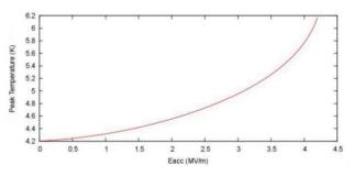
Figure 5: peak temperature of the membrane versus the accelerating field in the cavity (no dissipation in the seal).
