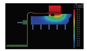
Figure 7: thermal simulation result. The blue arrows represent the liquid helium cooling.
