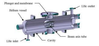
Figure 1: the IFMIF HWR prototype.
