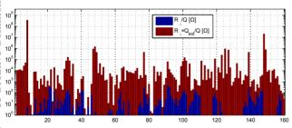
Figure 4: Transverse  $R/Q_{\perp}$  and  $R/Q_{\perp} \cdot Q_{\text{ext}}$  for all TM and TE modes up to 2.85 GHz (beginning of 4<sup>th</sup> dipole band). The arrow marks the coupler kick by the TTF-III power coupler at the fundamental mode.
