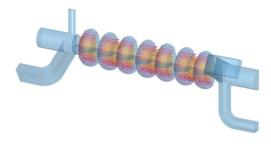
Figure 1: Rendering of the cavity design under consideration for B*ERL*inPro with a cut through the symmetry (FPC) plane and electric field magnitude of the operational mode.
