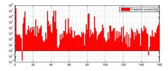
Figure 7: Approximate (orders of magnitude) calculations for the treshold current based on Eq. 4.
