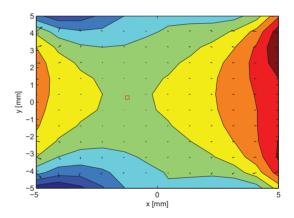
Figure 1: Reconstruction of the transverse (arrows) and longitudinal (isolines) voltages in the beam area with contributions from different multipole components. The corresponding coefficients were computed from voltages on circularly arranged integration paths at 5mm offset from beam axis for an eigenmode of the BERLinPro main linac cavity. The red square marks the transverse forceless point  $z_0$  which deviates from the axis by more than 1 mm.
