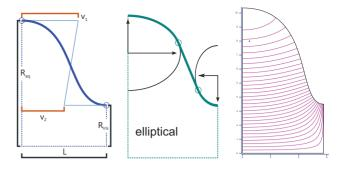
Figure 2: Parameterization for cubic Bezier shape (left), elliptical parameterization (center) and exemplary result for electric field lines ( $v_1 = 0.9, v_2 = 0.65, R_{\rm iris} = 35\,{\rm mm}, R_{\rm eq} = 103.60\,{\rm mm}, {\rm right}$ )
