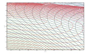
Figure 3: Cubic Bezier map for a 1.3 GHz cavity with iris radius 35 mm. The map shows the cubic interpolated isolines of  $R/Q[\Omega]$  in black,  $E_{\rm surf}/E_{\rm acc}$  in red, the Geometry factor  $[\Omega]$  in green, and the intercell coupling constant  $[10^{-3}]$  in blue.
