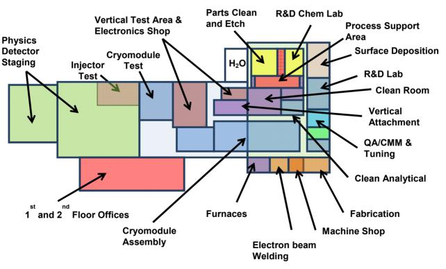
Figure 1: Overview schematic of new Test Lab/TEDF SRF facilities at Jefferson Lab, to be complete summer 2013.
