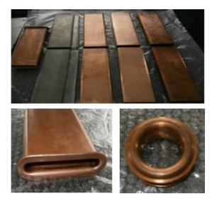
Figure 8: Parts of copper CH cavity.
