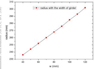
Figure 4: The radius of CH cavity with the width of girder.
