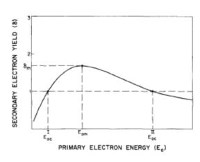
Figure 1: Definition of secondary-electron yield-curve parameters [6]
