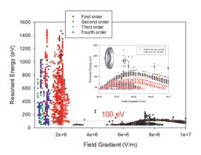
Figure 5: Resonant electron impact energy in region 1 for gradients up to 10 MV/m. The inset shows the impact energies for stable multipacting electrons for two different end cap outer rounding radii.
