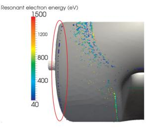
Figure 3: Resonant electrons and their impact energies surviving after 50 rf cycles as simulated by Track3P.
