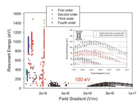
Figure 7: Resonant electron impact energy in region 2 for gradients up to 10 MV/m. The inset shows the impact energies for stable multipacting electrons for two different rounding radii where the spoke base meets the outer conductor.
