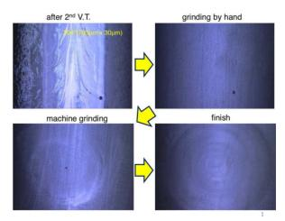
Figure 14: The progresses on the local grinding effect. The defect detected by the optical inspection was removed by the treatment.
