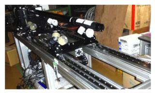
Figure 3: Latest CavCam-3 for SPL cavity at CERN.
