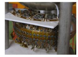
Figure 7: Installed XT-map leaves on a cell.
