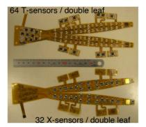
Figure 6: Leaf shaped flexible PCB.
