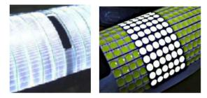
Figure 2: Enhanced illumination for wider surface area (Armadillo Illumination). 28 LED chips (right) instead of 2 LED's per strip (left) are installed.
