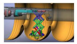
Figure 13: The grinding head assembly that has a tiny monitoring camera protrudes by a motor control towards the area to be treated.
