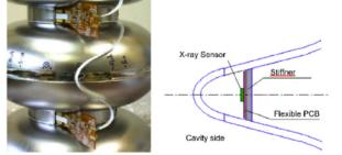
Figure 9: Installed stiffener X-map ribbons. The ribbons go under the stiffer ring.
