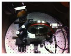
Figure 11: Layout for the laser induced X-ray radiography experiment. Various target materials can be irradiated by the laser to generate X-rays.
