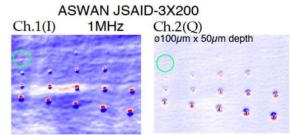
Figure 10: The high resolution eddy current scanner can detect the drilled holes on the Nb sheet down to  $ø100\mu$ m x 50  $\mu$ m depth.
